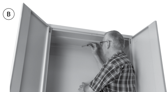
Fasten to the Back Panel with 3 x screws. Then, use a screwdriver to push the 'push-through' slots shown at 'A' into the Front Panel.
